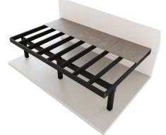
Add approximately 23mm for the deck surface (Check exact dimensions with supplier). Composite, tiles and turf + baseboards can be used for all deck heights. Hardwood for structures over 100mm high.
